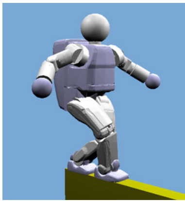
Fig. 6 The centroidal momentum-based controller can maintain postural balance of the humanoid robot under various disturbance forces
